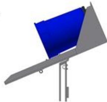
**Dumping Stations: 6 total stations; 3/4" Plywood construction, steel pivot hinges, black pipe handle. U-bolt attachment to field perimeter**
